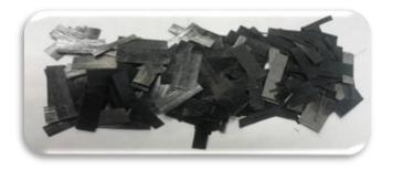
PMT-FormX consists of continuous prepreg slit and chopped into a randomly distributed array of material. The molding compound is preformed into a charge of specific shape and weight.
