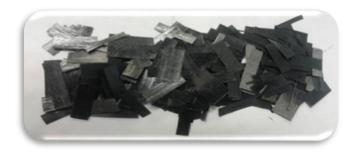
PMT-MC consists of continuous prepreg slit and chopped into a randomly distributed array of material. The molding compound is pre-formed into a charge of specific shape and weight.
